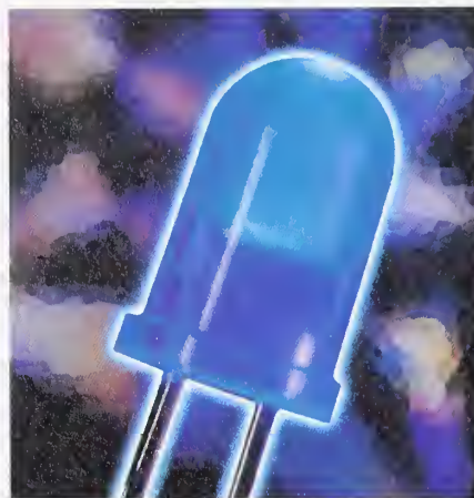
The low-cost blue light emitting diode (LED) produced with new silicon carbide crystal technology.
